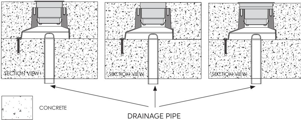
SOFT SOIL - Arrange an adequate water drainage system with pebbles.
