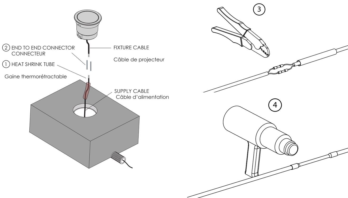
When connected, roll up the cable inside the formwork and put the fixture into the formwork itself.
