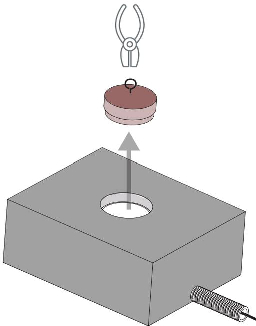
Before installing the fixture, remove the cap from the formwork by using pliers.
