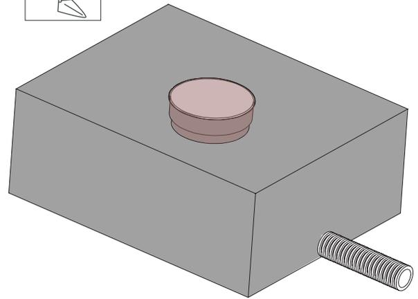
Fill with cement up to the level of the cap and clean off any material in excess that may prevent the removal of the cap
