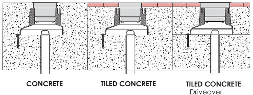
ATTENTION: To facilitate the removal of the cap, its recommended to use a release agent for formworks.
