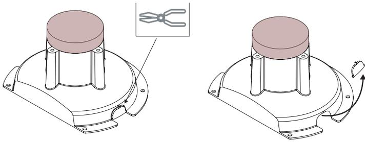
Insert the pipe into the formwork and then fix it to the ground through the specific fixing holes.
